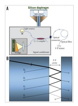
**Figure 4.** Fibre-optic pressure sensing technology. A) Fabry-Pérot white-light interferometer and coupler. B) A small fraction of the incident beam escapes the interferometer creating a large number of parallel beams of light. Reproduced with permission from Pinet<sup>3</sup>.
