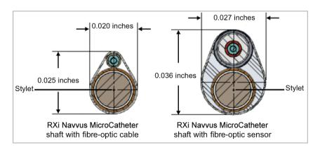
**Figure 3.** Profile and structure in cross-sectional view of the Navvus microcatheter at the level of the fibre-optic sensor and at the lesion site. At the level of the fibre-optic sensor the microcatheter has an elliptically shaped profile with dimensions of  $0.027" \times 0.036"$ . At the lesion site the profile of the microcatheter decreases to  $0.020" \times 0.025"$ ; these dimensions could be considered comparable to those of a 0.022" circular-shaped wire.
