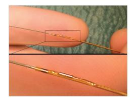
**Figure 2.** The Navvus Rapid Exchange system and profile. Upper panel: Navvus MicroCatheter system with a standard wire (BMW) showing the profile of the microcatheter. Lower panel: magnification of the tip of the microcatheter with the fibre-optic sensor.
