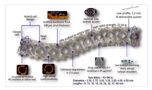
Figure 1. Design of the MeRes100 bioresorbable vascular scaffold stent platform.
