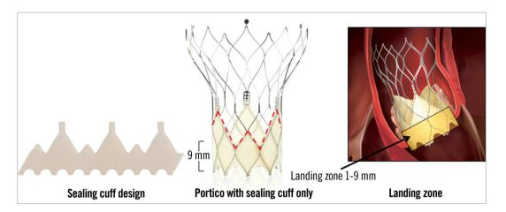
**Figure 19.** *St. Jude Portico*<sup>TM</sup> *TAVI device. Details of the sealing cuff design and height determining a target landing zone between 1 and 9 mm below the aortic annulus.*
