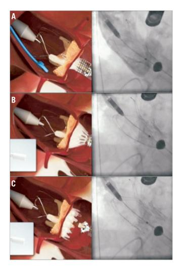
**Figure 22.** ACURATE  $TA^{TM}$  implantation. A) Implantation step 1. The prosthesis is partially unsheathed releasing the stabilisation arms and the upper crown of the stent body. B) By pulling on the system the operator will get tactile feedback, the delivery system will embrace the native calcified leaflets and the upper crown will compress the tissue. C) The stent body is fully deployed and self-detaches from the delivery system.
