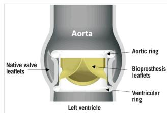
Figure 16. Direct Flow Medical<sup>®</sup> valve in situ.
