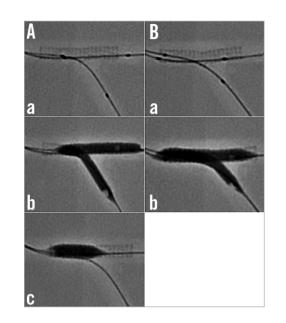
**Figure 1.** Bench comparisons of minimal (MBO) versus long (LBO) balloon overlapping during KBI. A) MBO. a) Location of 3.5 and 3.0 mm balloons in the bifurcation model, where a 3.5 mm stent was deployed in the MV; b) simultaneous inflation; c) proximal MV dilation with a 4.5/8 mm balloon. B) LBO. a) Location of 3.5 and 3.0 mm balloons; b) simultaneous inflation.
