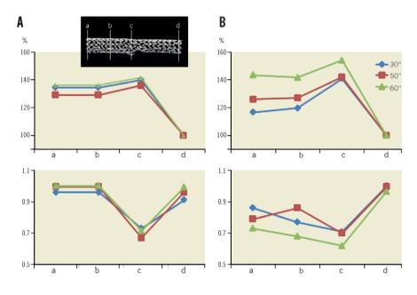
**Figure 5.** Comparison in cross-sectional area and eccentric index of the stent after KBI with MBO and LBO with bifurcation angle at 30, 50, and 60 degrees. A) Percent change of cross-sectional area at proximal edge (a), middle point of the proximal part of the stent (b), carina (c), and distal edge (d). Left: MBO. Right: LBO. The area at the distal edge of the stent was regarded as 100%. B) Eccentric index. Note that similar stent expansion was obtained by MBO.
