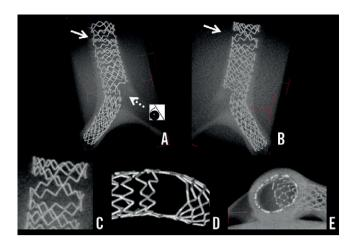
**Figure 6.** Images of Endeavor stent with 2-link connection deployed in a 3-dimensional Y-shaped model. A) View from the top. B) View from the bottom. C) Magnified view of overdilatation of the proximal struts outlined by the arrows in panels A) and B). D) Magnified view of the LCX ostium, after complete removal of the jailed struts, from the vantage point shown by the dotted arrow in panel A). E) Cross-sectional view from the inner side at the bifurcation.
