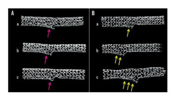
**Figure 3.** *MFCT images of stent configuration after KBI with bifurcation angle at 30 (a), 50 (b), and 60 degrees (c). A) MBO. B) LBO. Note the difference in the stent deformation at the SB. More deformation was observed according to the bifurcation angle in LBO (yellow arrows) compared to a similar change in MBO (pink arrows).*
