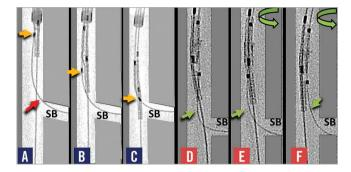
**Online Figure 1.** Bench testing sheds light on stent delivery problems. Wire bias in panels A-C directs the side branch component (yellow arrow) of a two-wire dedicated bifurcation stent away from the side branch (SB) preventing rotation and delivery. In panels D-F, a torquable shaft facilitates rotation and alignment with separation of wires (green arrows) making delivery possible.
