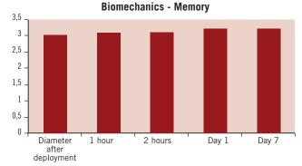
Figure 2. Graph showing the learning process of the PLA stent resulting in a slight, 5% increase of the stent diameter (Y axis, in mm) one hour after in vitro deployment, and 10% after 2 hours of in vitro deployment. This results, without recoil, at 7 days.
