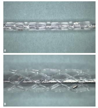
Figure 1. A. PLA stent gently crimped on the balloon resulting in neither strut cracks nor crazing; B. PLA expanded stent deployment presenting neither strut cracks nor crazing.
