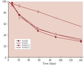
Figure 4. Graphs showing the evolution of the resorption of various PLA stereoco-polymer films in vitro (right) and explanted PLA stents in vivo (left) (Y axis: percentage of molecular weight) at various time-points (X axis: time in days). Comparison of the 2 graphs demonstrates the good relationship between our in vitro and in vivo models.
