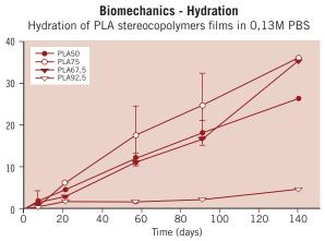
Figure 3. Graph showing the evolution of the hydration of various PLA stereoco-polymer films (Y axis: percentage of hydration) throughout time (X axis: time in days).
